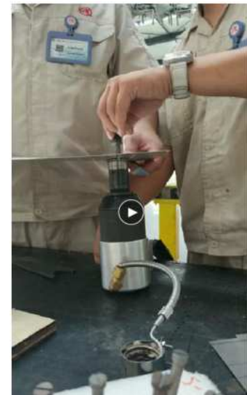
Figure 3. ZT2021D Blind Pull Gun Portable Dimpler being used.
