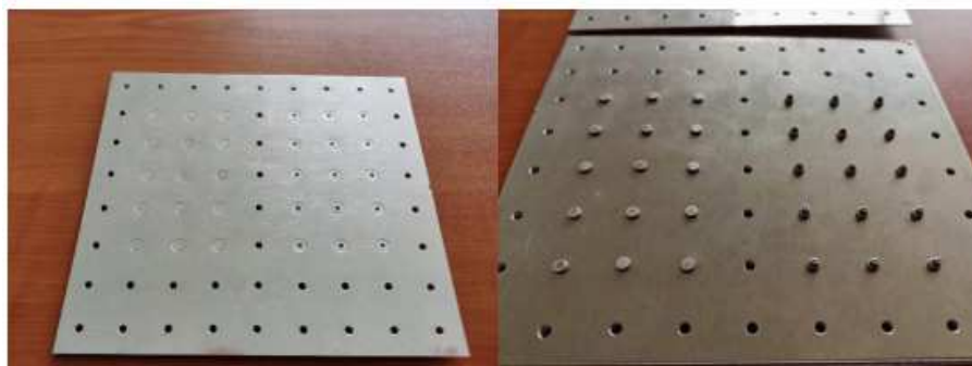
Figure 7. Rivet head and upset head after riveting of aluminum plate.
