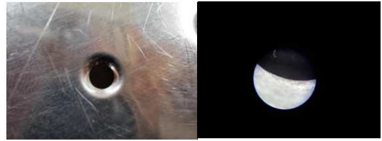
Figure 9. 60x magnifier of the dimple.
