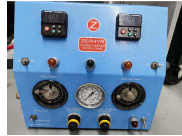
Figure 1. ZT2409G Thermo Dimpler Control Panel.
