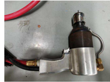
Figure 2. ZT2021D Blind Pull Gun Portable Dimpler.
