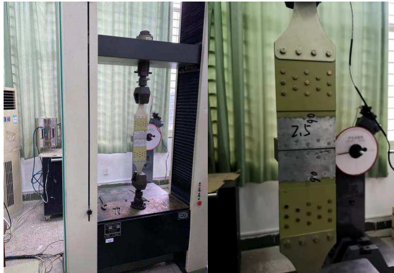
Figure 10. Specimen installed on tension machine.
