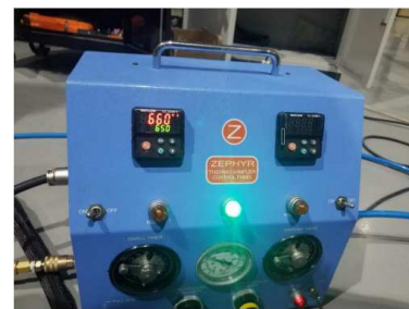
Figure 6. The temperature controller sets the dimpling temperature at 343°C (650°F).
