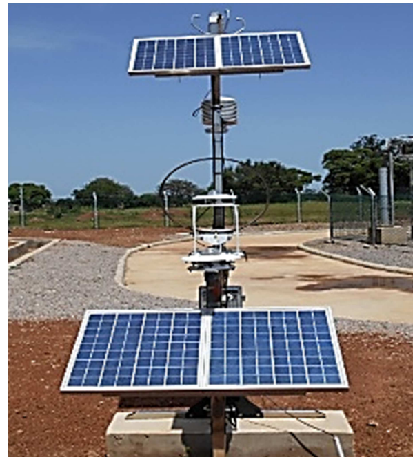
Figure 5. Solar PV Powered Meteorological Station.
